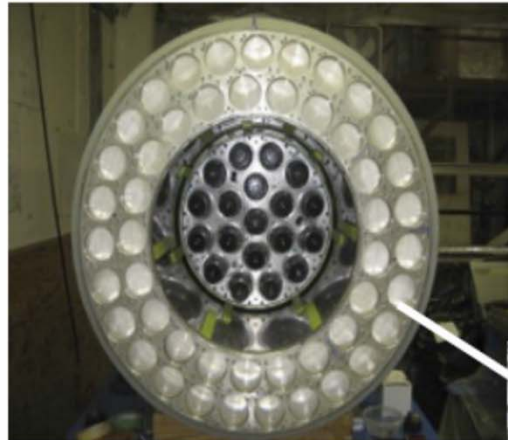
Monolithic NaI(Tl) crystal surrounded by 97 pure CsI crystals
