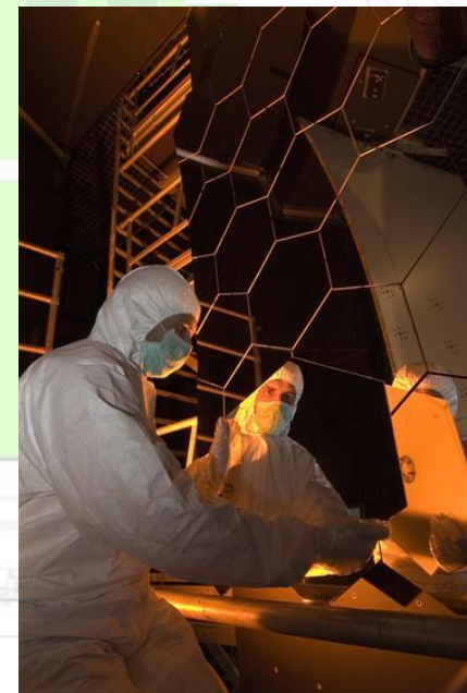
Assembling RICH 2; note the mirrors
