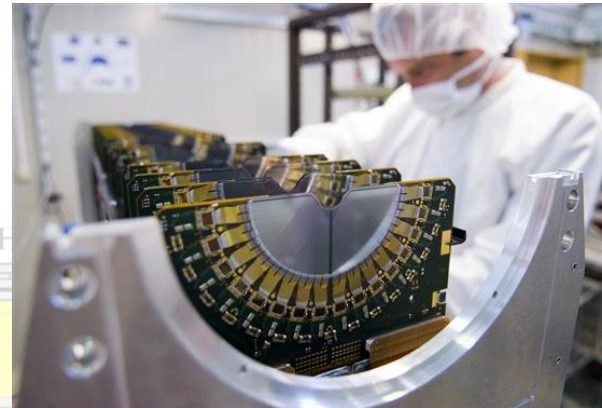
One-half of the VELO under construction
